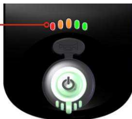
The battery gauge
