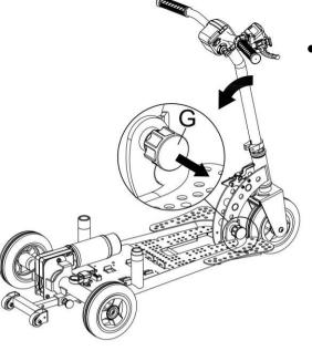
Use one hand to hold the handle, and use the other hand to pull the lock pin knob (G) and turn it anticlockwise. Then fold the handle down until you hear the "click" of the locking pin fitting into position on the main frame.
