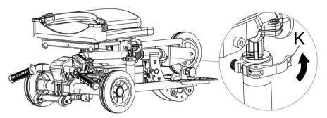
When the seat is folded and positioned on the scooter, the seat post clamp "K" must be tightened securely.
