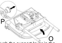
Push the support lever in the direction of the arrow until it clicks into position "**R**".
