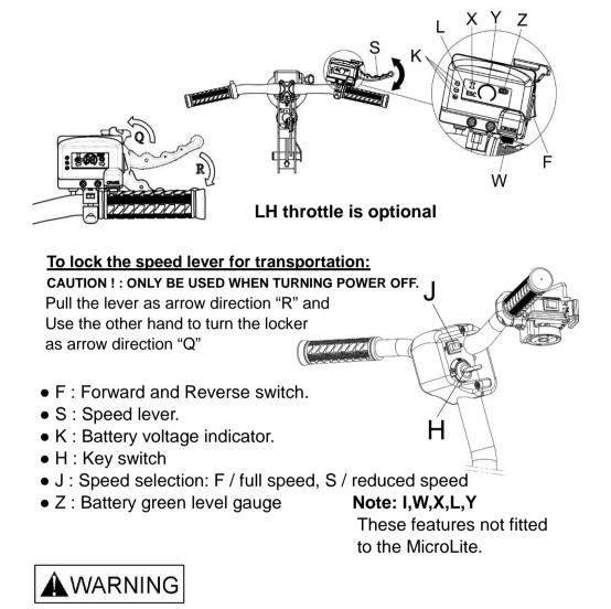
Do not place your fingers on the speed lever before you turn the key switch "On".
