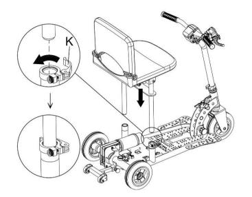
• Insert the seat frame tubes into the corresponding holes on the main frame, and then tighten the lever clamp "K" as illustration.
