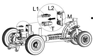
Press the lock tab of connector and pull out to disconnect the connector as per illustration.
