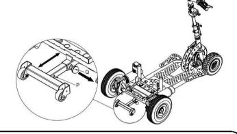
WARNING ! To prevent the scooter from tipping backwards the anti-tip frame must be locked in the maximum extended position.
