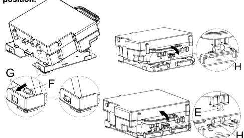
• To move the battery just pull up and move away.
