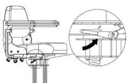
To turn the seat, lift and hold the release handle below the seat (as shown). This will allow the seat to turn.
