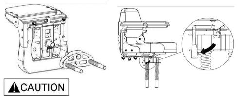
When removing the seat, do not lift the release handle as this could cause the seat support frame to disconnect from the seat and fall.
