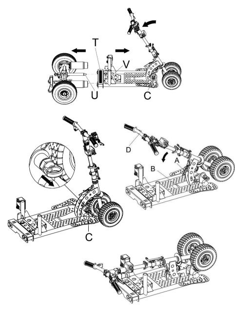
• Use one hand to hold the handle, and use the other hand to pull the lock pin knob (C) and turn it anticlockwise. Then fold the handle down until you hear the "click" of the locking pin fitting into position on the main frame.
