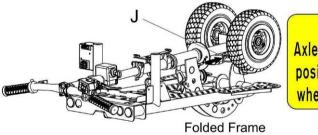
WARNING ! Axle must be securely locked in position after assembling front wheels. (Refer to user manual)
