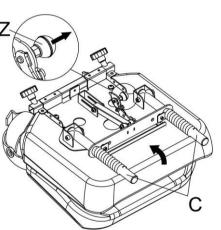
Push the support lever in the direction of the arrow until it clicks into position "E". Warning: Pin "E" must be locked into the position before using.
