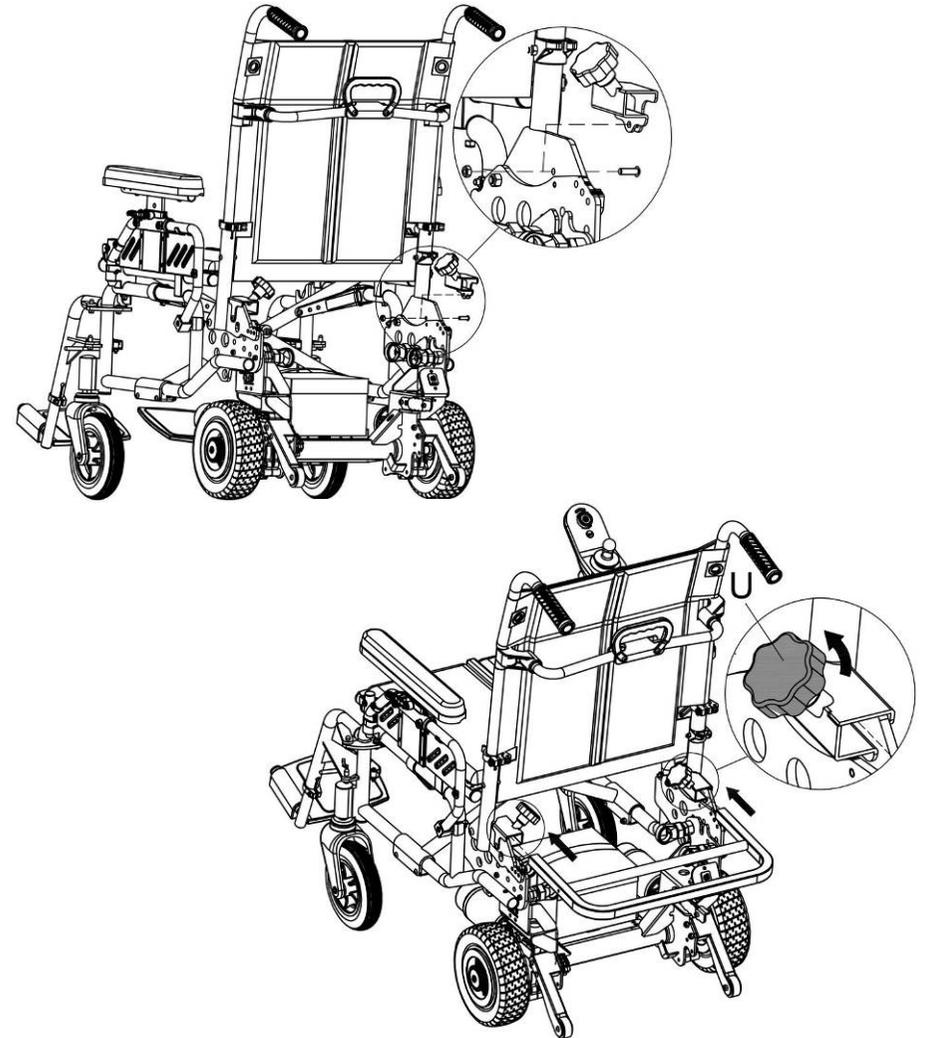
Assemble the luggage frame per illustration and tighten bolt "U".
