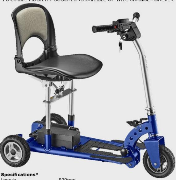
Length 930mm Width 500mm Max Load (Level Ground ) 100kg Max Speed 6kph 8 - 10km Est. Travel Range 175 x 50mm Tyre Sizes (Solid) Battery (Lithium) 24v 8.7ah Motor 230w Total Weight 18kg Weight minus Seat and Battery 11.8kg Front Basket
