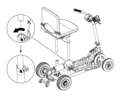
• Insert the seat frame tubes into the corresponding holes on the main frame, and then tighten the lever clamp "K" as illustration.
