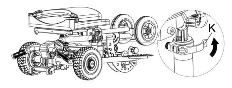
When the seat is folded and positioned on the scooter, the seat post clamp "K" must be tightened securely.
