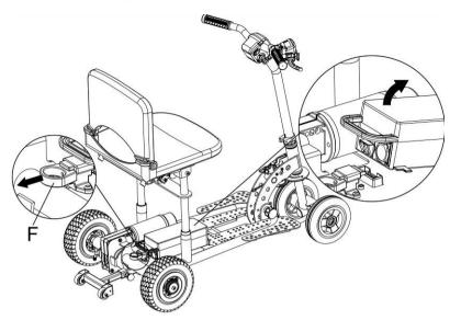
• Use one finger to pull the ring "F", and use the other hand to pull the battery pack upward and then move the battery module away from scooter.
