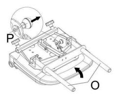
Push the support lever in the direction of the arrow until it clicks into position "R".
