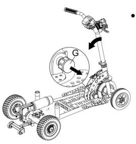
• Use one hand to hold the handle, and use the other hand to pull the lock pin knob (G) and turn it anticlockwise. Then fold the handle down until you hear the "click" of the locking pin fitting into position on the main frame.
